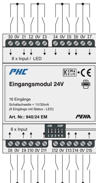
On 0 V port (earth) is intended for each 2 button inputs. The 0 V ports are internally connected in the module. It needs to be ensured that the button is operated with the earth of the module to which they are connected.
